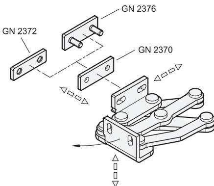
The Stainless Steel-Multiple-joint hinges can be adjusted in three planes during installation. For example, this allows tolerances to be adjusted or the required compressive forces for seals to be established. Two planes can be adjusted via the parallel or perpendicular slots in the fixing angle pieces. In the third plane, position corrections can be made using the Stainless Steel-Spacer plates GN 2370 (see page).
